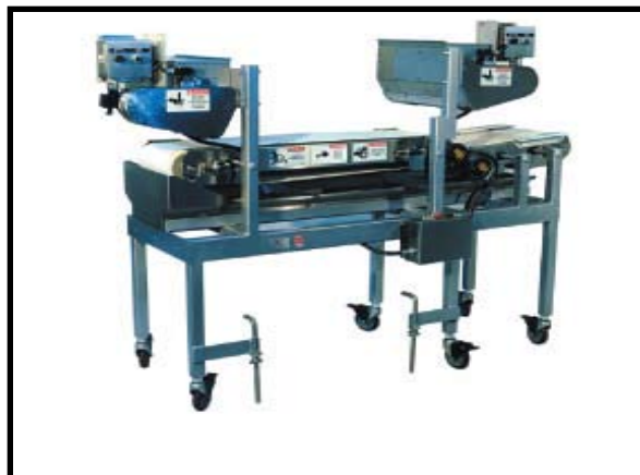
Single Channel Flouring and Outfeed Conveyor for Use With Cone Rounder
